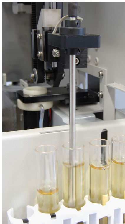
Throughput: up to 120 samples per hour. The sample volume is 2.0 ml.
