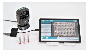
PlatR lets users import or prepare their pipetting plans and navigates their pipetting on microtiter plates by illuminating the wells according to the plan.
